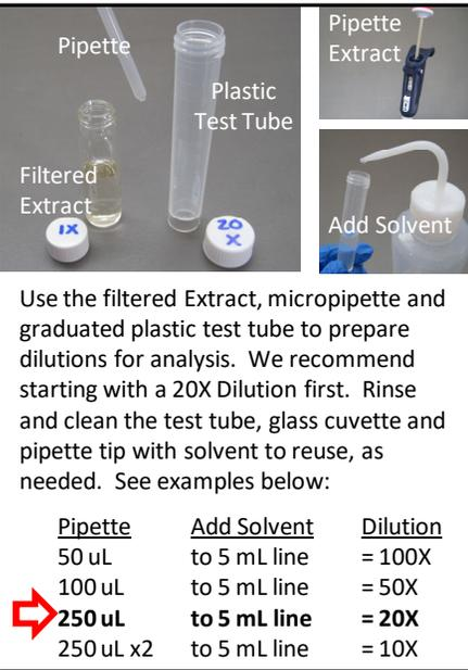
Use the filtered Extract, micropipette and graduated plastic test tube to prepare dilutions for analysis. We recommend starting with a 20X Dilution first. Rinse and clean the test tube, glass cuvette and pipette tip with solvent to reuse, as needed. See examples below:
