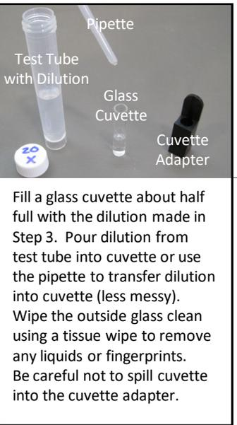
Fill a glass cuvette about half full with the dilution made in Step 3. Pour dilution from test tube into cuvette or use the pipette to transfer dilution into cuvette (less messy). Wipe the outside glass clean using a tissue wipe to remove any liquids or fingerprints. Be careful not to spill cuvette into the cuvette adapter.
