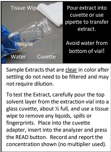
Pour extract into cuvette or use pipette to transfer extract. Avoid water from bottom of vial!
