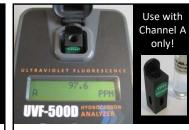
The UVF-500D includes a 100 ppm TPH Solid Standard. This device was specially 'tuned' to read the same as the 100 ppm Calibrator used in CAL-056H-500D when the analyzer was factory calibrated. If its available, test the TPH Solid Standard after a new calibration is performed. If readings are close to 100 ppm (within +/- 10%), the Solid Standard is accurate/performs well
