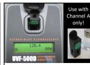
The UVF-500D includes a 100 ppm TPH Solid Standard. This device was specially 'tuned' to read the same as the 100 ppm Calibrator in CAL-056H-500D (in hexane solvent) when the analyzer was factory calibrated. If its available, test the TPH Solid Standard after a new calibration is performed. Readings should be higher, typically 10-20%, and consistent each time it's used.
