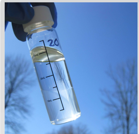
Samples are extracted in graduated 40 mL glass VOA vials using 15 mL of water with 15 mL solvent and then analyzed on the UVF-500D.
