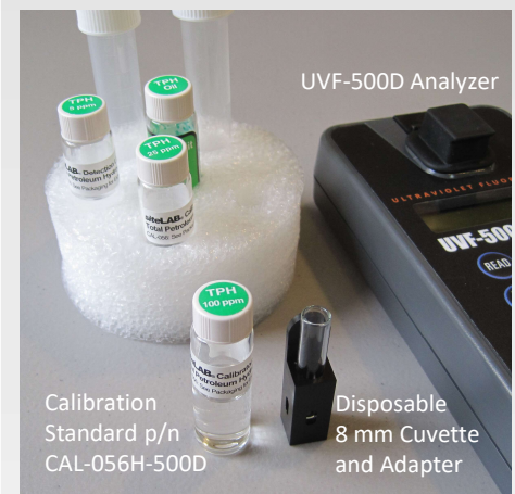
Samples are extracted in graduated 40 mL glass VOA vials using 15 mL of water with 15 mL solvent and then analyzed on the UVF-500D.
